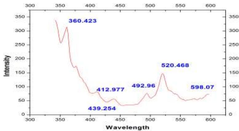
Figure 5.1: PL spectra of Pure ZnO Nanoparticles
