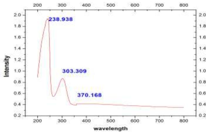
Figure 4.2: Optical absorption spectra of Al doped ZnO Nanopowder
