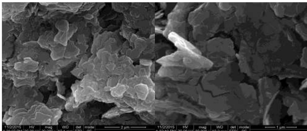
Figure 2.2 :SEM Pictures of Al Doped Pure ZnO nanoparticles
