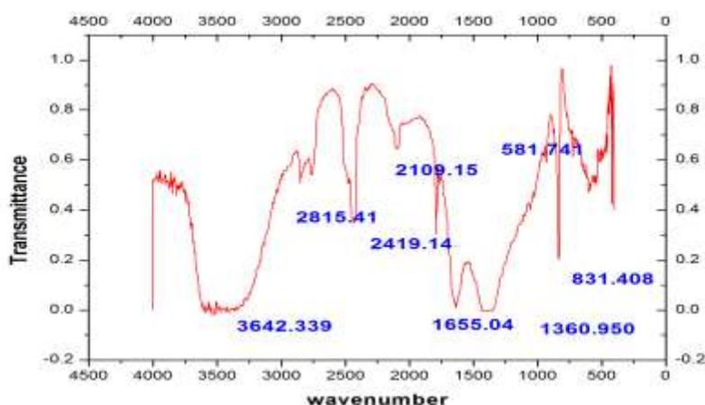
Figure 3.1: FTIR spectra of Al doped ZnO Nanopowder
