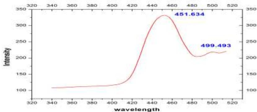
Figure 5.2: PL spectra of Al doped ZnO Nanopowder
