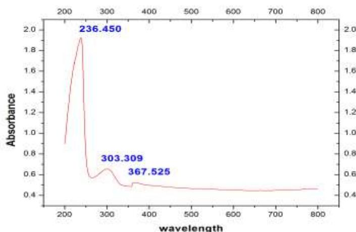
Figure 4.1: Optical absorption spectra of Pure ZnO Nanopowder
