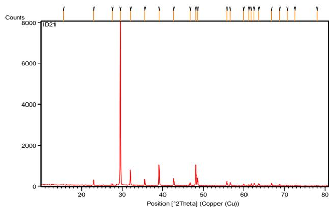
Figure 1.2: XRD Spectra of Al doped ZnO Nanoparticle
