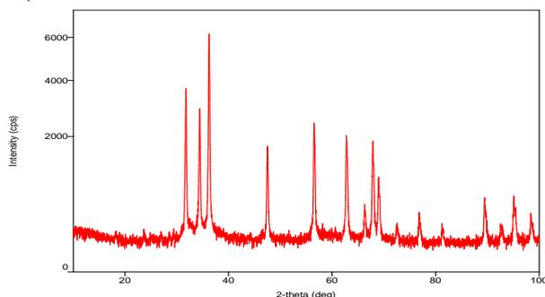
**Figure 1.1:** XRD Spectra of Pure ZnO Nanoparticle
