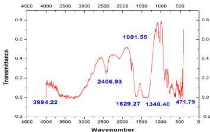
Figure 3.1: FTIR spectra of Pure ZnO Nanopowder
