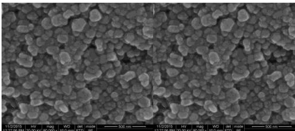
Figure 2.1: SEM Pictures of Pure ZnO nanoparticles
